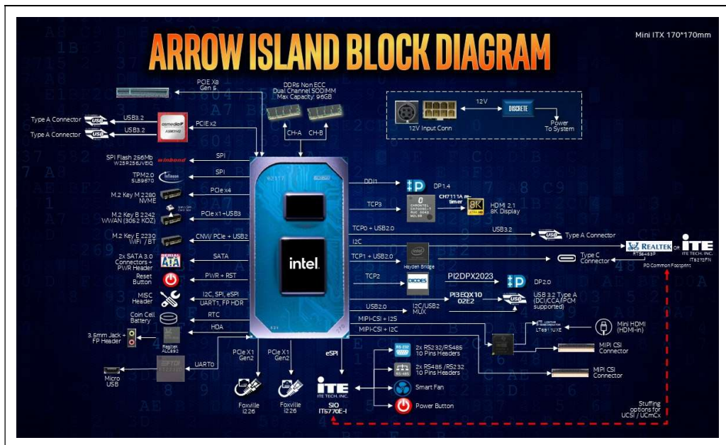
Figure 1. Block Diagram of the Evaluation Kit
