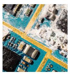
contact with water, electrical conductivity increases and the process speeds up. Any acid will corrode the metal even faster.
